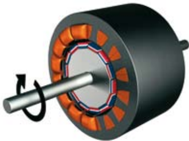
Internal rotor motor with 15 grooves and 14 surface magnets
