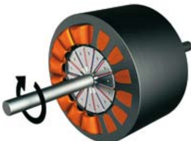
Internal rotor motor with 15 grooves and 14 embedded magnets, 'spoke design'
