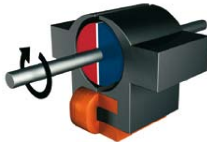
Single-phase motor with bipolar ring magnet
