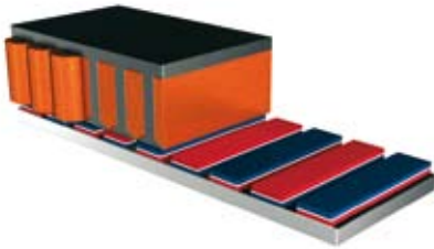
Linear motor with 6 grooves and n magnets
