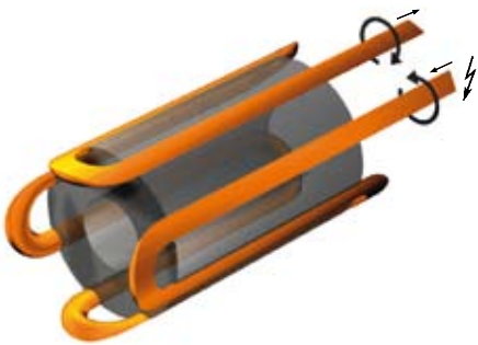
Magnetisation coil for 8-pole magnetisation on the inside diameter
